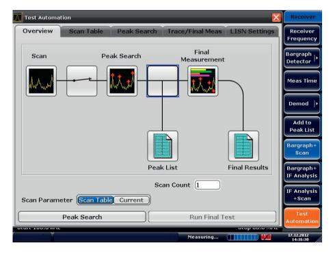
The R&S<sup>®</sup>ESRP allows users to configure automatic test sequences (preview measurement, data reduction, final measurement) quickly and easily and execute them at the press of a button. The final measurement can also be carried out interactively.
